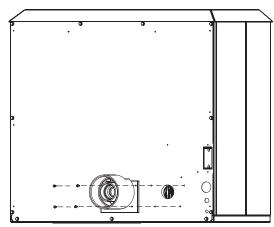
**Step 2.** Attach co-axial direct vent adaptor and gasket (4 screws) to the rear of fireplace.
